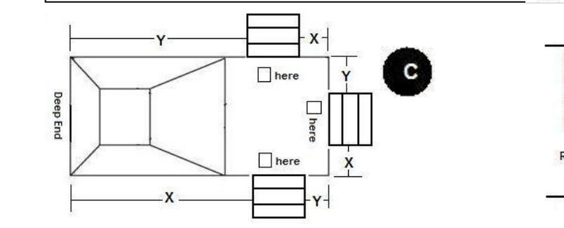
**D Depth and Width: Measure the total step width and depth. Note that the depth includes the recess.**
