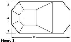
Referring to the illustration of your grecian pool (figure 1), be sure that the width (A) and the length (B) measurements are made at the bead receiver (where the liner snaps into the track), not at the edge of the coping (the edge of the pool
