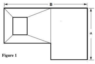
Referring to the illustration of your True-L pool (Figure 1), be sure that the width (A) and the length (B) measurements are made at the bead
