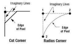
Measure the diagonals from the squared corners. If the corners of your pool are rounded (radius) or cut (diagonal), be sure to measure to squared corners. Refer to the diagram (Figure 5) for instructions on measuring to squared corners. **Record all measurements in the MEASURING FORM.**
